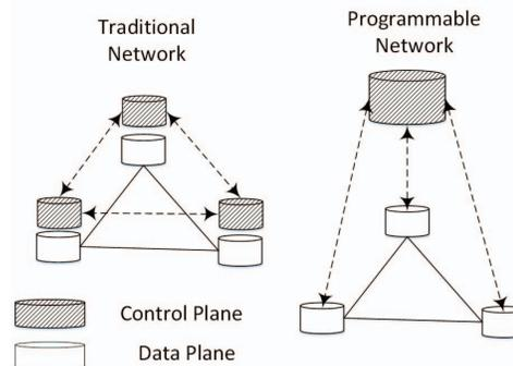
Fig. 1. Difference in Control Plane implementation in traditional and programmable networks
