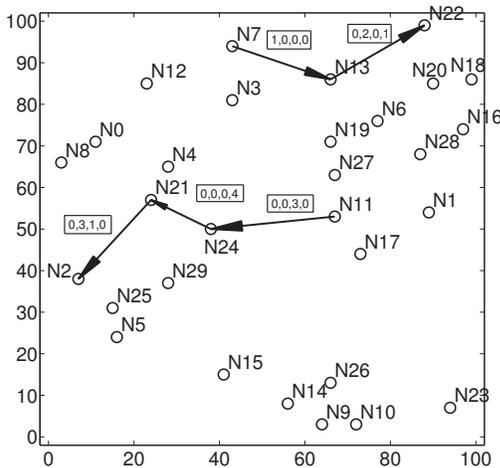
Fig. 5. Shows the combined results for all time slots (with the number of data streams for each time slot on the link shown in a box).
