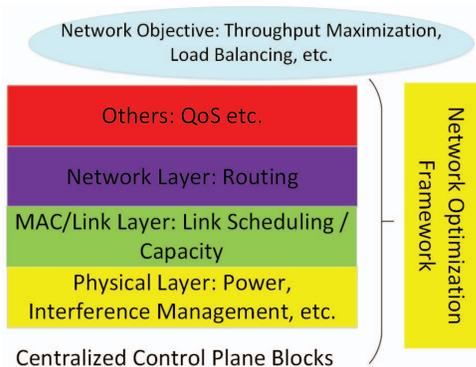
Fig. 2. Wireless Programmable Control Plane Building Blocks
