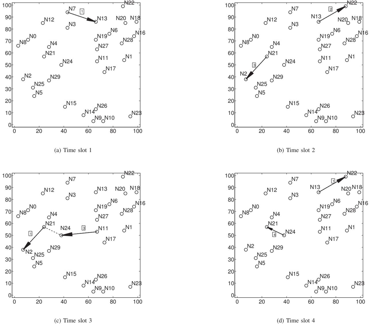
Fig. 4. Scheduled links, DoFs allocation on each link, and interference pattern in time slots 1 to 4, respectively.
