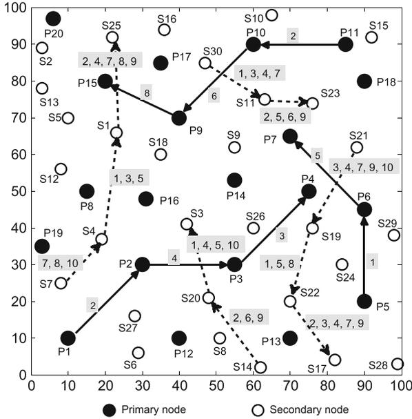
**Fig. 7** Channel allocation on each link for the secondary sessions. Channel allocation on each link for the primary sessions is given a priori
