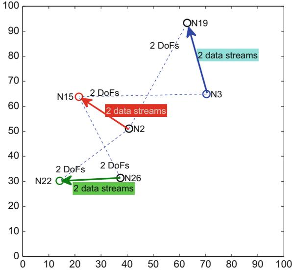
**Fig. 3** The DoF allocation in the optimal solution in band 1 for the 30-node CRN<sup>MIMO</sup> example
