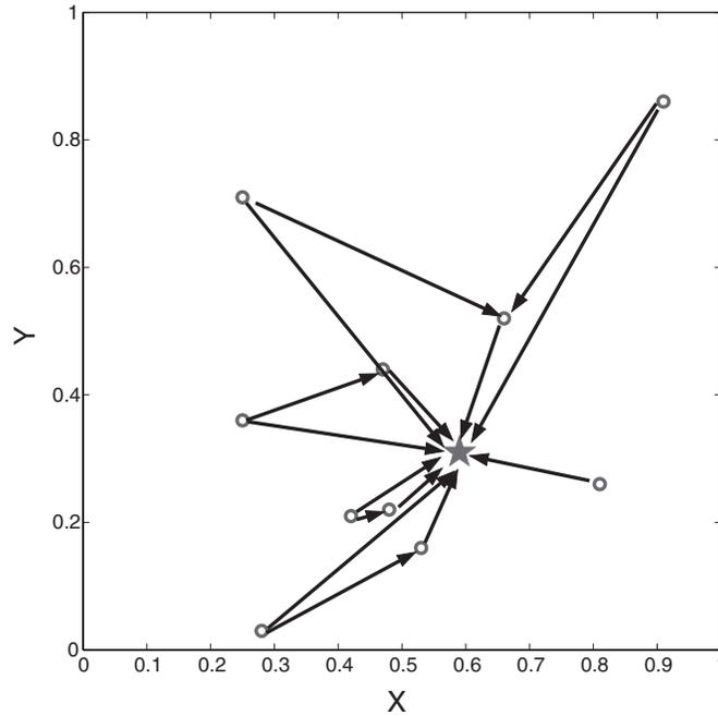
Fig. 5. A schematic showing the routing solution for the 10-node network with base station being placed at (0.59, 0.31).
