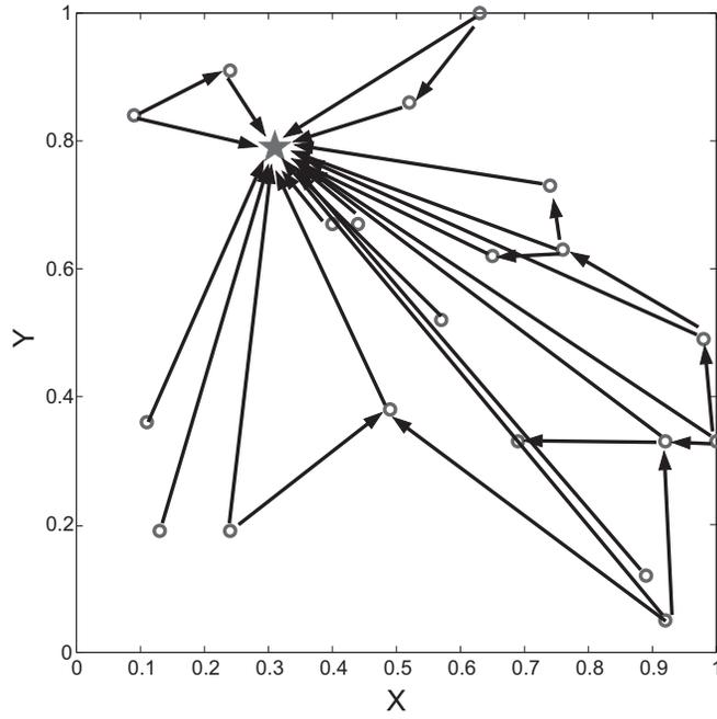
Fig. 6. A schematic showing the routing solution for the 20-node network with base station being placed at (0.31, 0.79).
