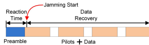
Fig. 5: Extended frame structure
