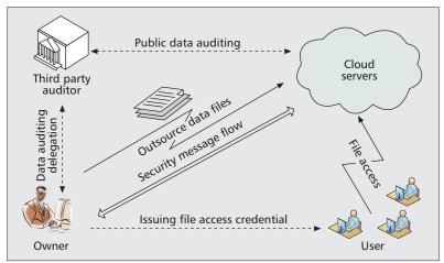
Figure 1. The architecture of cloud data storage service.
