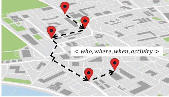
Fig. 1. Illustration of mobile tracking. Location data samples are collected and stored by MNOs. We define a data sample as a mobility event in the format of a quadruple \langle who, where, when, activity \rangle . MNOs can compile the data samples into user trajectories and further make data inferences using any available tools like artificial intelligence.
