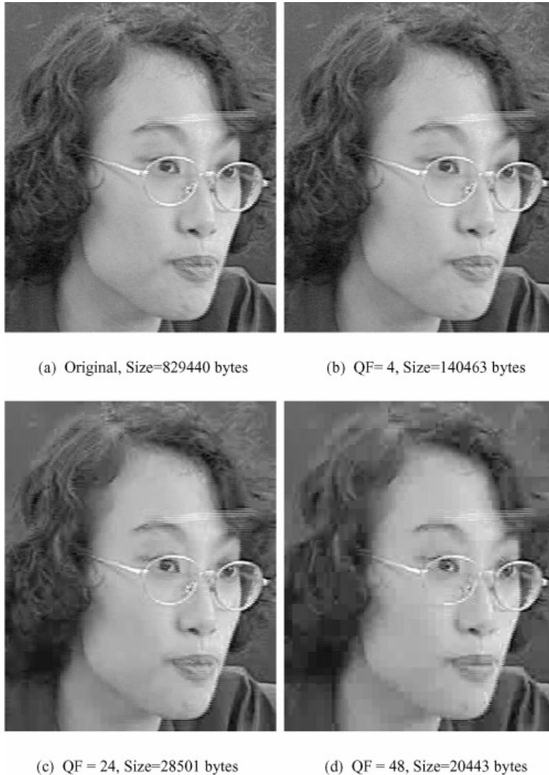
Figure 2. Effect of quantization factor on picture quality.
