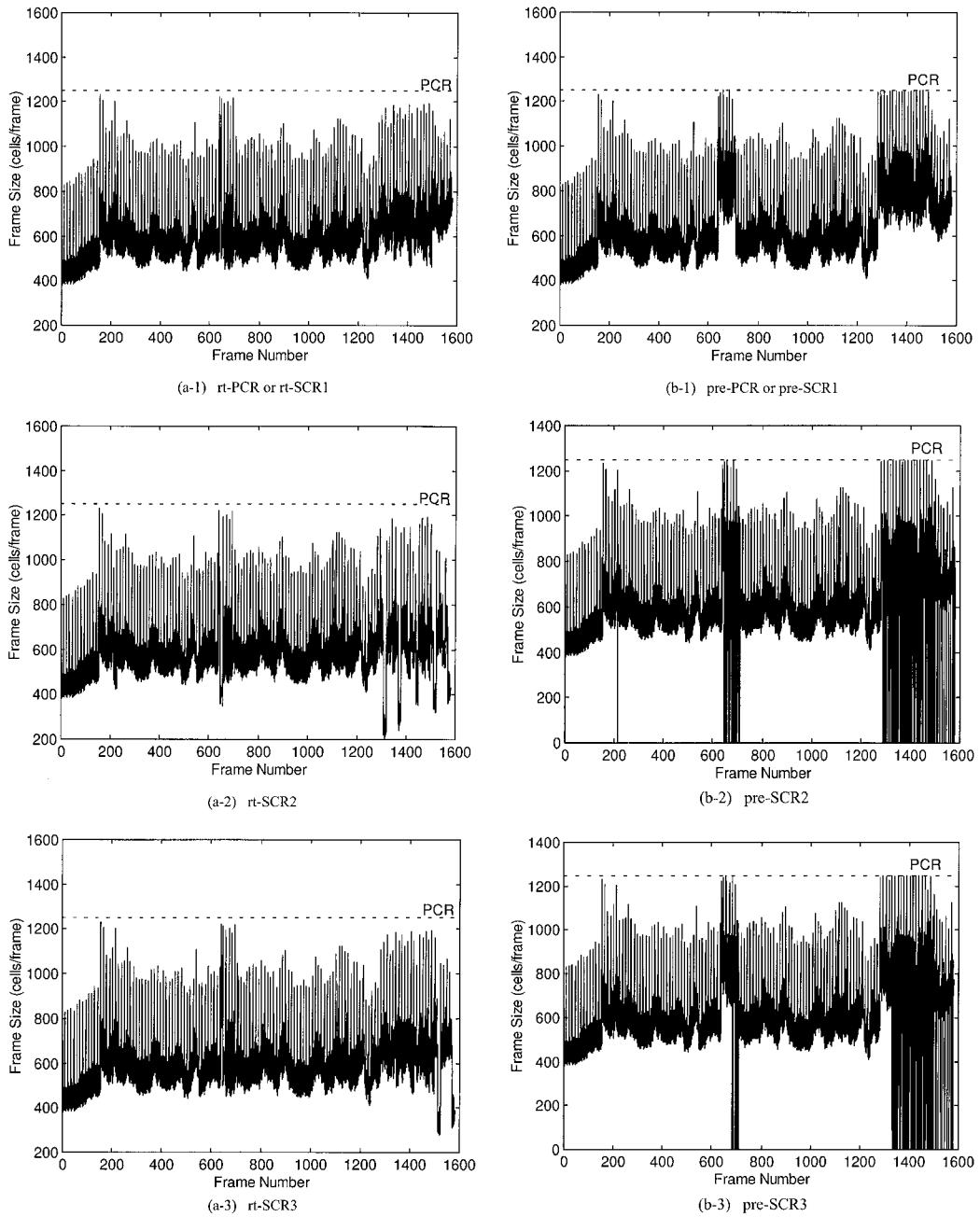
Figure 7. Cells per frame time series (controlled VBR).
