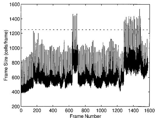
Figure 6. Cells per frame time series (pure VBR).
