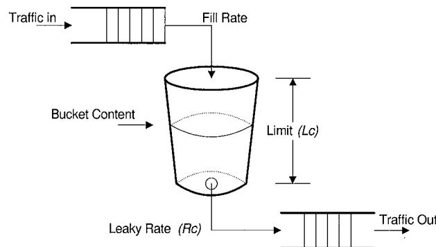
Figure 1. Modified leaky bucket algorithm model.
