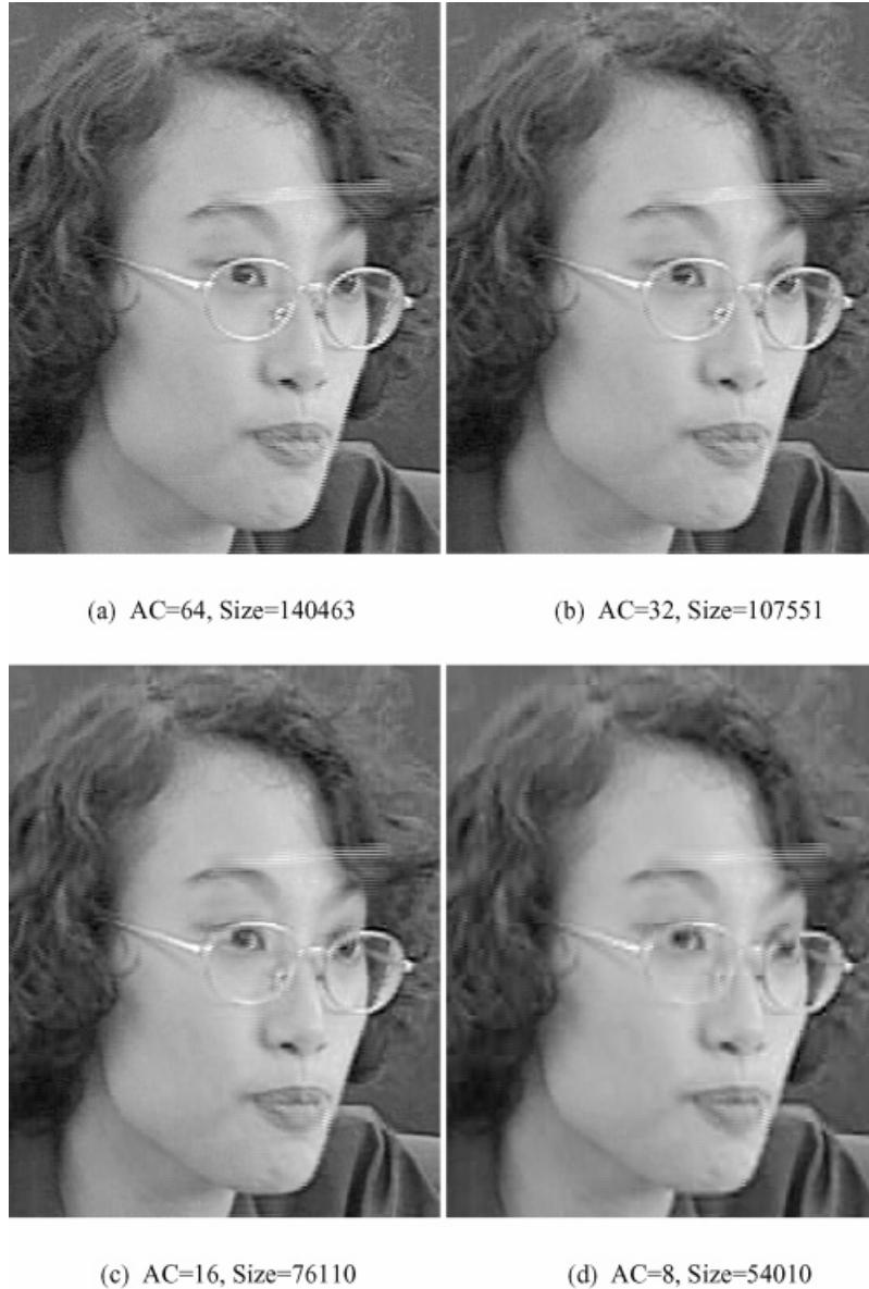
Figure 5. Effect of number of AC coefficients on picture quality.
