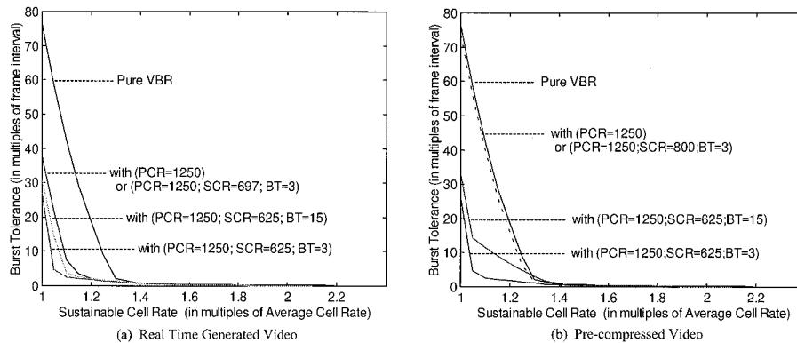
Figure 10. Usage parameters for lossless transmission.
