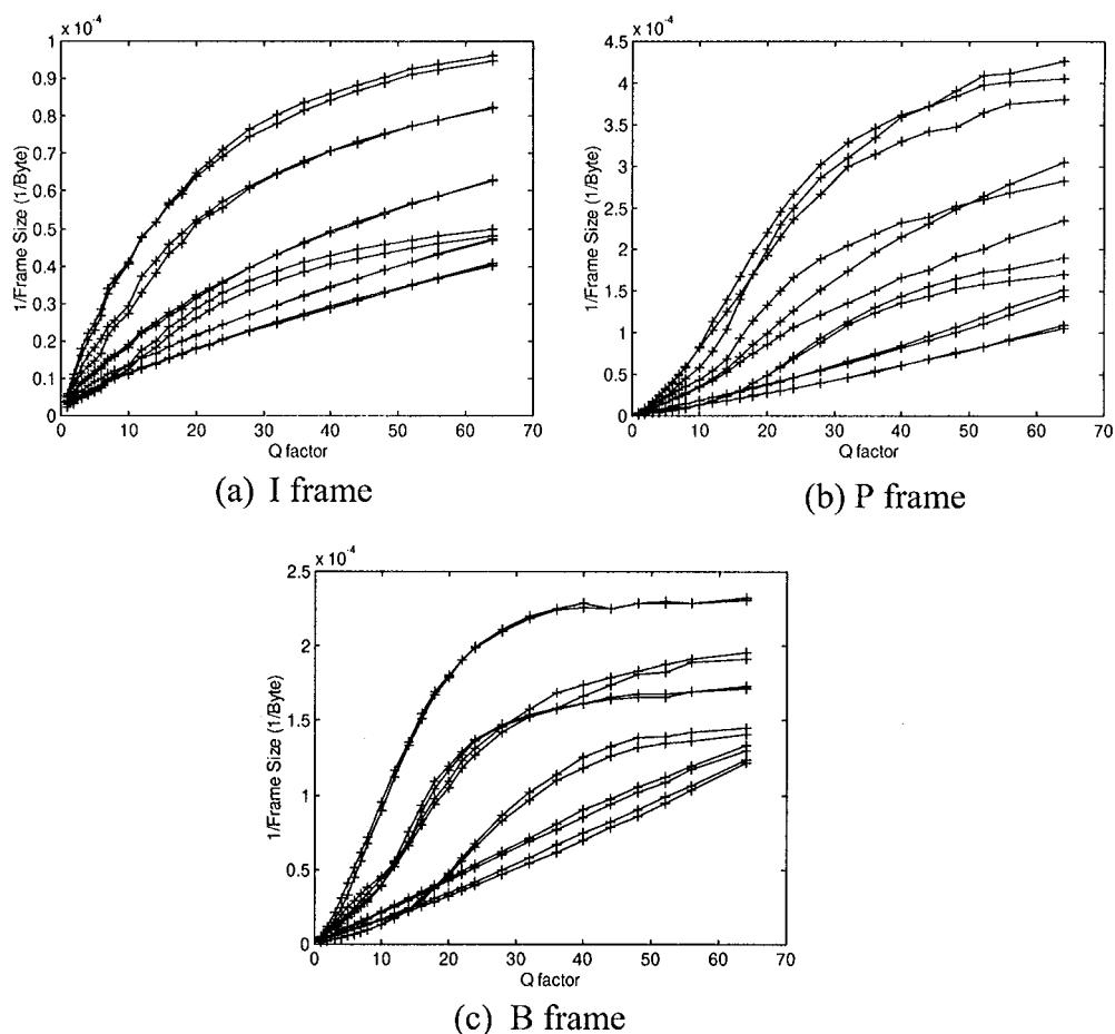
Figure 3. The relationship between quantization factor and frame size.
