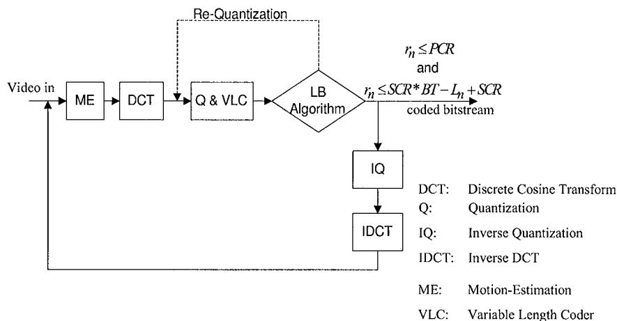
Figure 4. UPC-based MPEG encoder structure.
