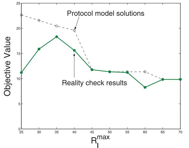
Fig. 3. Protocol model solutions and corresponding reality check results for the 20-node 5-session network.
