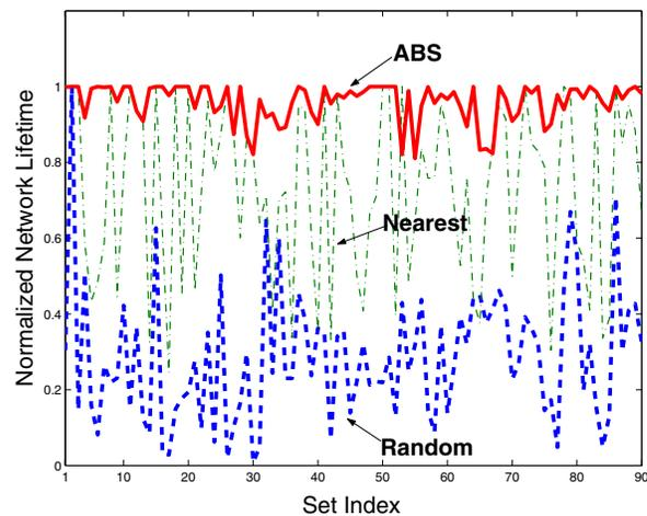
**Figure 2. The normalized network lifetimes under the ABS, Nearest, and Random base station selection for 90 data sets.**
