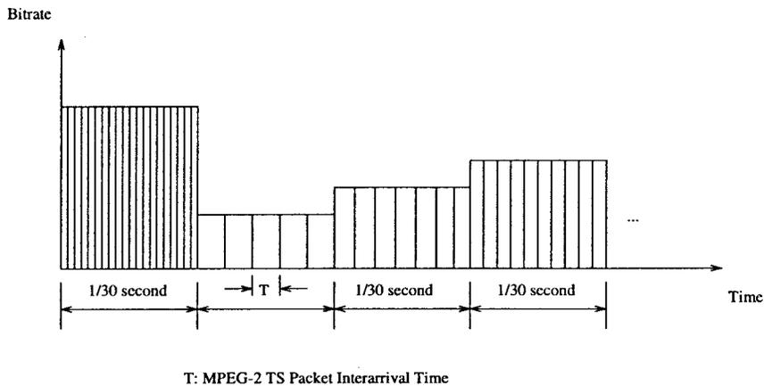
Fig. 1. MPEG-2 transport packet generation process.
