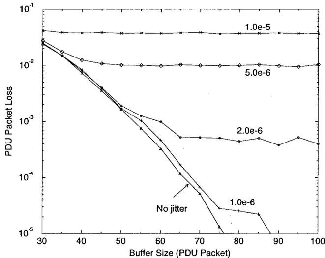
Fig. 3. Relations among packet loss ratio (due to packet late arrivals and buffer overflow), buffer size, and jitter level. The number above each curve specifies the variance of the PDU packet jitter simulated.
