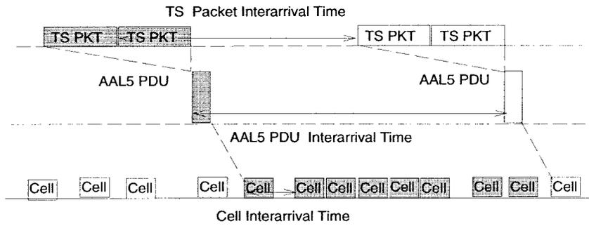
Fig. 2. The process of reassembling eight ATM cells into an AAL5-PDU.
