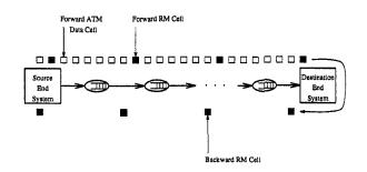
Figure 2: Rate-based closed-loop flow control for an ABR virtual connection.
