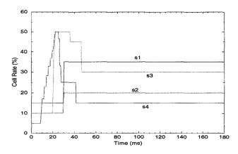
Figure 5: The cell rates of all connections for the WMM policy in the parking-lot network configuration.
