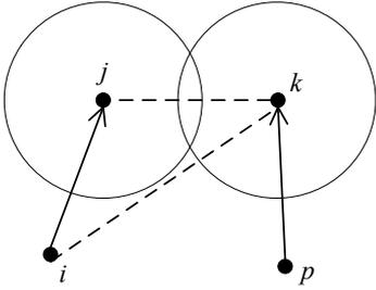
Fig. 1. Overlapping of two circular footprints of two receiving nodes.
