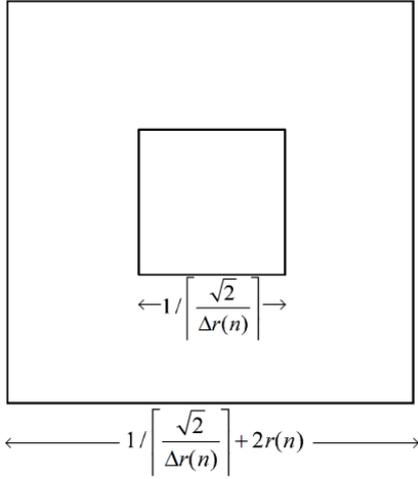
Fig. 5. The larger square contains all the transmitters that can transmit directional beams to the receivers that are in the small interference square at the center.
