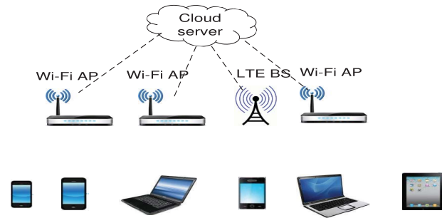
Fig. 2. A cloud-based control plane that coordinates spectrum sharing between Wi-Fi APs and LTE BS.
