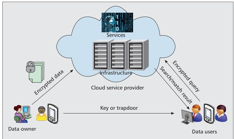
Figure 1. System architecture for searchable cloud data storage services.
