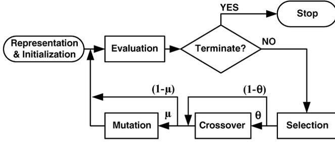
Fig. 4. Flow chart of the GA-based approach.
