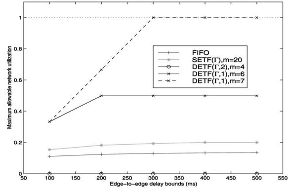
Fig. 11. Provisioning power of FIFO, SETF( $\Gamma$ ), DETF( $\Gamma, 1$ ), and DETF( $\Gamma, 2$ ) networks ( $H^* = 8$ ).
